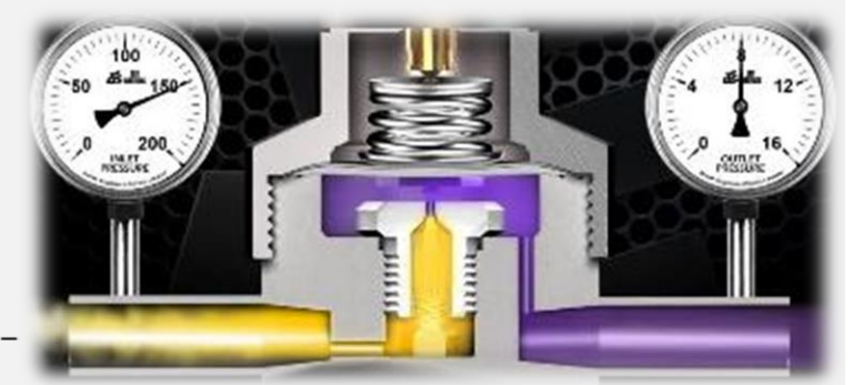
Pressure reduce by passing through a controlled small orifice.
