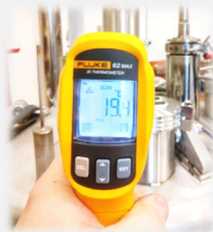
Checking the delta between outer Jacket and temperature ambient.
